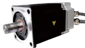
80 Series Direct-Output Wire DC (Brake) Servo Motor Rated voltage: 48V Rated power: 750W Rated torque: 2.4Nm Rated speed: 3000rpm
