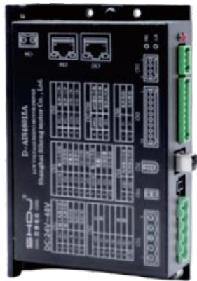
Driver AiBH2-4805C Voltage output range: 24-48V Rated current: 5A Compatible motors: 20/28/42/57/60 series three-phase closed-loop stepper motors Communication: RS485/CANopen/EtherCAT
