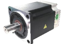
80 Series DC (Brake) Servo Motor Rated voltage: 48/72V Rated power: 750/1000W Rated torque: 2.4/3.2Nm Rated speed: 3000rpm
