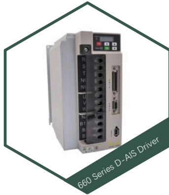
D-AIS38050A AC Servo Drive Input Power: 380V Module Current: 50A Compatible motors: 110/130 series Position control / Speed control / Torque control / Communication control pulse / Analog signal / 485 / CANopen / EtherCAT
