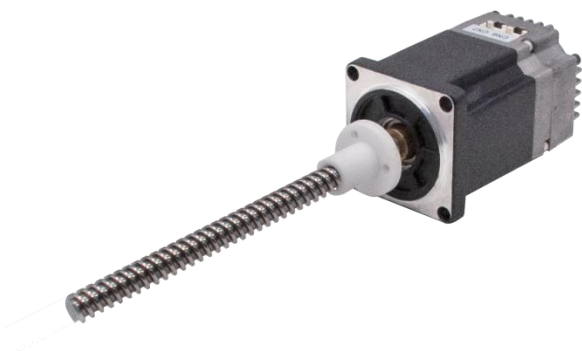
60AIS Series DC Servo Screw Rod Motor Rated voltage: 24/48V Rated Power: 31/62/94W Screw Rod Diameter: 14/15.875mm Lead Screw Pitch: 2/3/4/6/10/12/18mm 2.54/3.175/5.08/12.7/25.4mm
