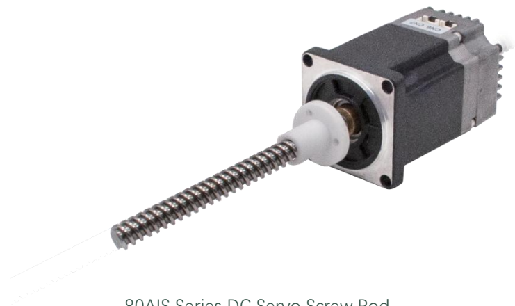
80AIS Series DC Servo Screw Rod Motor Rated voltage: 48V Rated Power: 750/1000W Screw Rod Diameter: 16/20mm Lead Screw Pitch: 2/4/5/10/16/25mm
