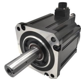
180BST Series AC (Brake) Servo Motor Rated voltage: 220V/380V Rated power: 2.9/4.5kW/5.5kW/5.8kW/7.5kW Rated torque: 18.6N/28.4N/35N/48N Compatible driver: D-AIS22050A/D-AIS38050A
