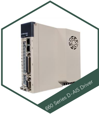
D-AIS22020A AC Servo Drive Input Power: 220V Module Current: 20A Compatible motors: 40/60/80 series Position control / Speed control / Torque control / Communication control pulse / Analog signal / 485 / CANopen / EtherCAT
