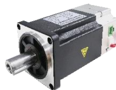
60 Series DC (Brake) Servo Motor Rated voltage: 24/48V Rated power: 200/400W Rated torque: 0.64/1.27Nm Rated speed: 3000rpm
