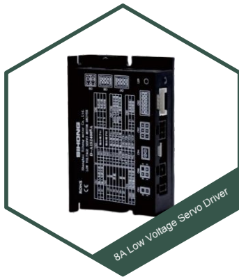
8A Low Voltage Servo Driver Rated Current: 8A Voltage Range: 24V~36V Position control, speed control, torque control, communication control Pulse/Analog/485/CANopen/EtherCAT
