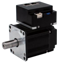
60 Series Backpack-Type DC (Brake) Servo Motor Rated voltage: 48V Rated power: 400W Rated torque: 1.27Nm Rated speed: 3000rpm
